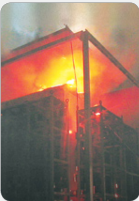
Fig.2 Arc test without arc duct (HMS -N12)
