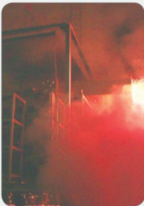
Fig.3 Arc test with arc duct (HMS-N12C)
